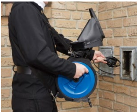
Fig. 30: Cable reel camera carried with carrying belt system
