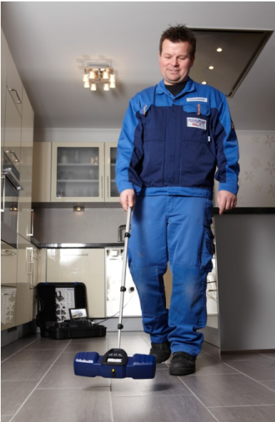
Fig. 15: Localizing the camera head underground
