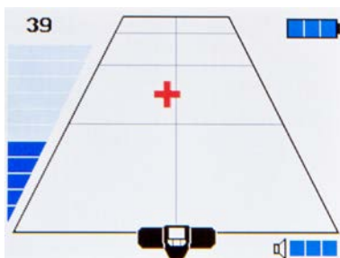
Fig. 14. Localizing the camera head
